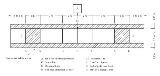
For foil and épée the conductive surface must cover the whole of the length and breadth of the piste, including its extensions (run back) and its safety borders (cf. Article t.13s, m.57)
