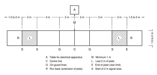
For foil and épée the conductive surface must cover the whole of the length and breadth of the piste, including its extensions (run back) (cf. Article t.13s, m.57)
